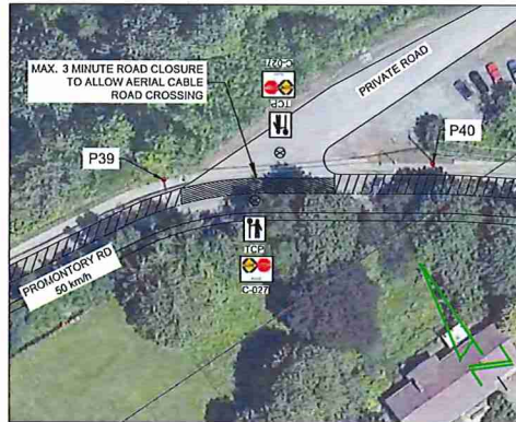
ROAD CROSSING FROM P40 TO P39
